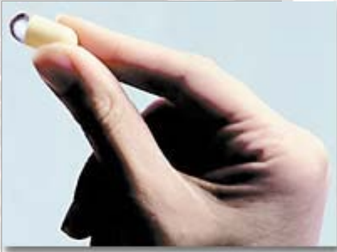
Figure 1. A wireless endoscopy system in a capsule provides real-color images of the GI tract after the patient swallows the device.
