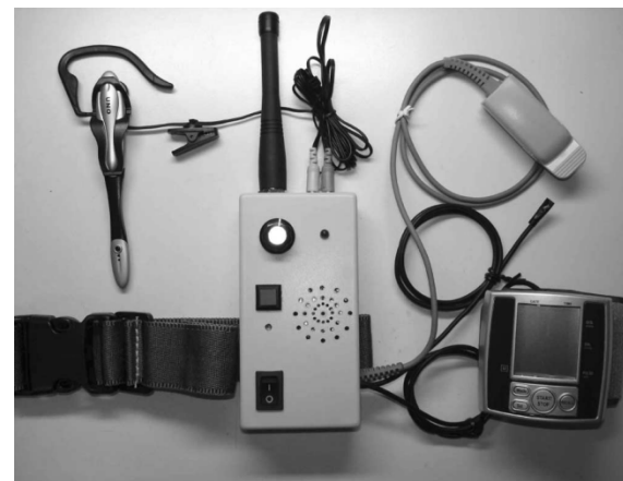
AMON (multiparameter monitor, wrist-worn device, EU-funded project)
