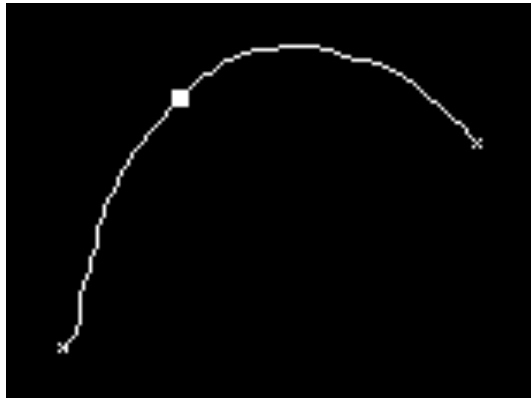
Isolation of a single ridge, its centroid, its end and start points
