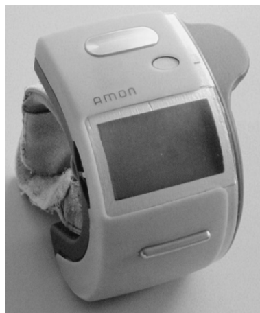
AMON (multiparameter monitor, wrist-worn device, EU-funded project)
